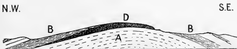
FIG. 48. Lenticular intrusion (phacolith) in anticline of Ordovician strata, Corndon, Shropshire, England. (After Lapworth and Watts.) A. Flags and shales; B. ashes and andesite; D. dolerite.
